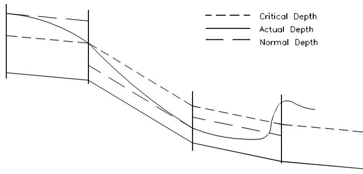
Trial 4, etc.: This process continues until the assumed and computed values of water surface elevation are within the allowable error tolerance. If they are, the computed water surface elevation becomes the converged solution.
